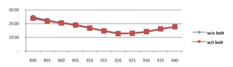
•STRIP reads same, with exactly the same sensitivity curve, regardless of whether it is fastened with metal bolt in two holes (located on both ends) or not. Stainless steel M3 bolt with round head is best fit for STRIP.
